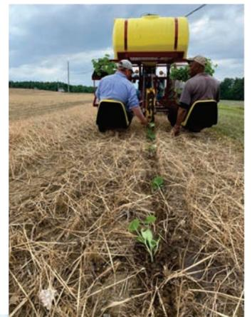
**Hydraulic lift No-till unit for P1500**, attaches on the P1500 3-point hook up instead of the hitch. Extremely easy to hook up and unhook to easily switch between no-till and conventional. Twin waved, spring loaded coulters and drip attachment. Call for pricing.
