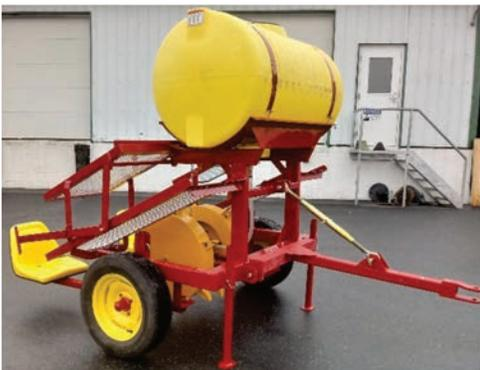
**P1500 Combination Pull-type** with large transport wheels, it converts easily to 3-point hook up by pulling 3 pins and dropping the hitch. Has adjustable turnbuckle on hitch for easy leveling. Same features as the P150, found on page 53. Ideal for those who want to use the no-till attachment in addition to their regular planting. Add \$125 inbound freight, **\$3,390.00**
