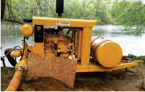
**Rainbow Pumps** the industry's best built engine pumps with John Deere or Isuzu diesel power units from 30 to 200 hp. Also available in electric VFD control. Engine pumps come with a murphy safety system monitor with auto shut down. Rainbow builds units with large fuel tanks and high-capacity radiators to prevent overheating. Quiet run type mufflers come standard, trailer or skid mount, and electric or protek primer. Please call for pricing and sizing per application.
