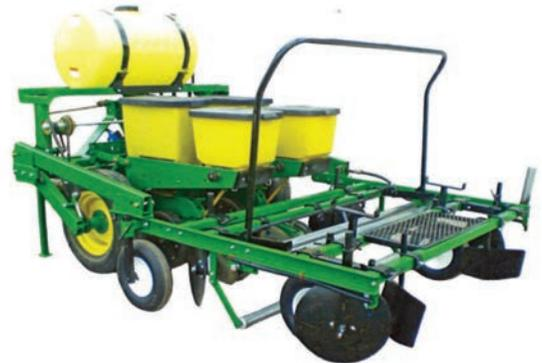
**Plants** 2 rows of sweet corn in furrows. 22" between rows. Between plant spacing 16"-30" and is easily adjustable. Uses John Deere 7000 series row units with precision planting finger meters, seed firmer and rubber closing wheels. The 2 furrow openers are 12" double discs that are adjustable in height with pin.
