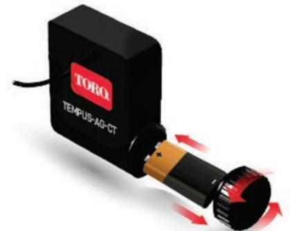
Tempus control units are powered by a 9V battery. The system will alert you when there is 20% battery life left. Only the base stations require 110 volt or a solar panel to create the network. No grid power is required to operate the system. When using irrigation control valves they have to operate with a 12 volt DC latching solenoid.
